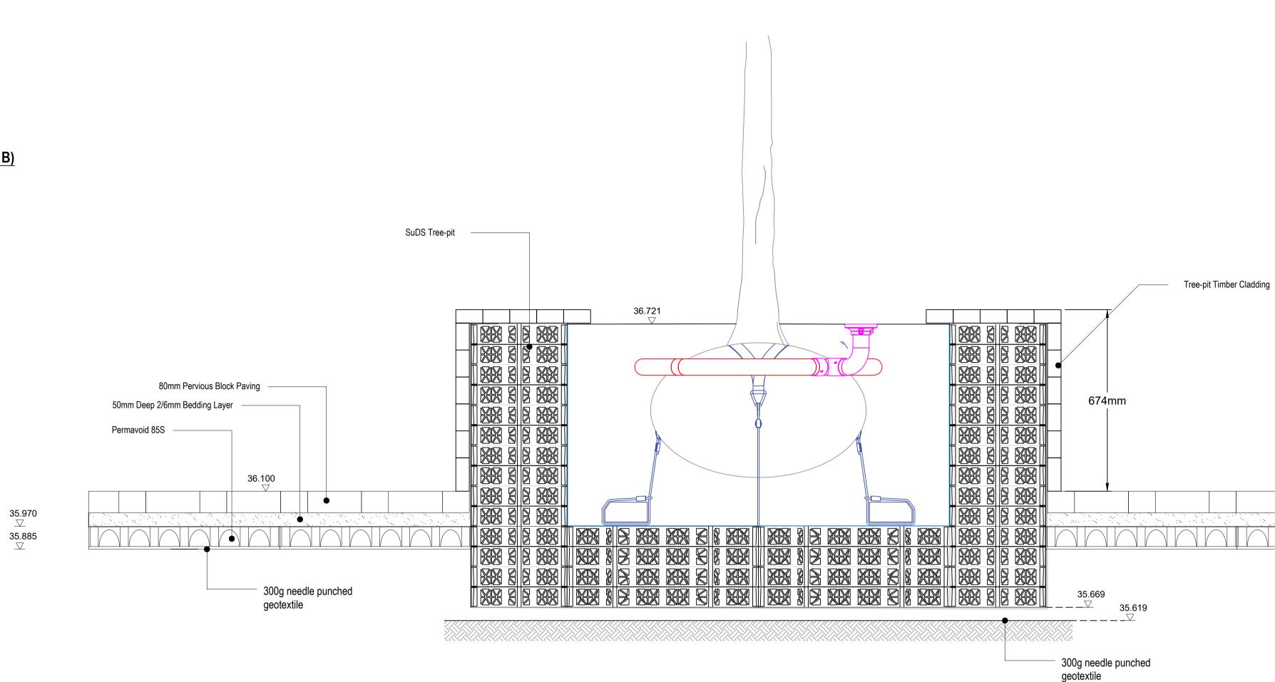
Section F-F: Section Through Shallow Open Water Feature (Area C)
