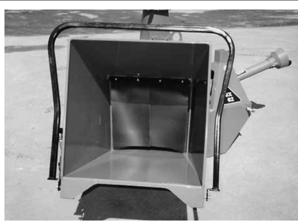
Example of curtain found in all BX model chippers
